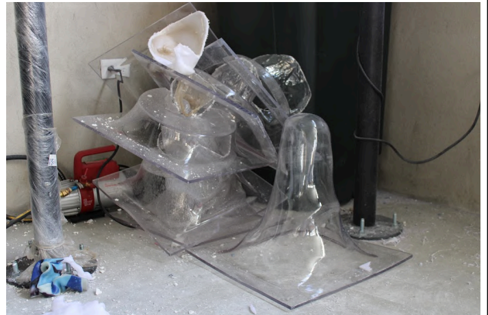
Test socket fabrication to improve the fit quality of prostheses.
